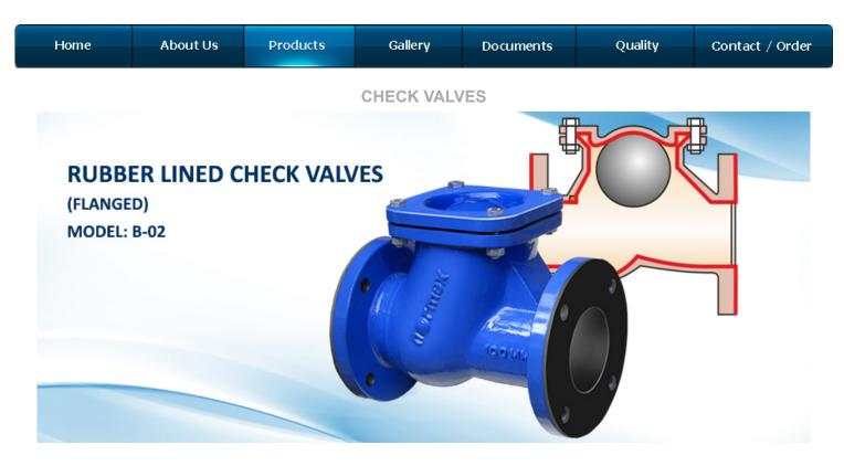
Rubber Lined Check Valves (Flanged) are lined internally with Ebonite Hard rubber so that media does not come in contact with metal. This Model is most suitable for corrosive/erosive applications. The overall dimensions of this valve will be similar to standard Ball NRV bur face. To face length will br more by 6-10mm.
