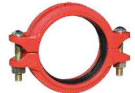
Style 1N Flexible Coupling DN25~DN300 1"~12" 33.4mm~323.9mm
